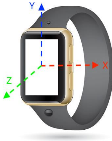
Figure 5.12. An illustration of accelerometer axes on a typical smartwatch is shown.
